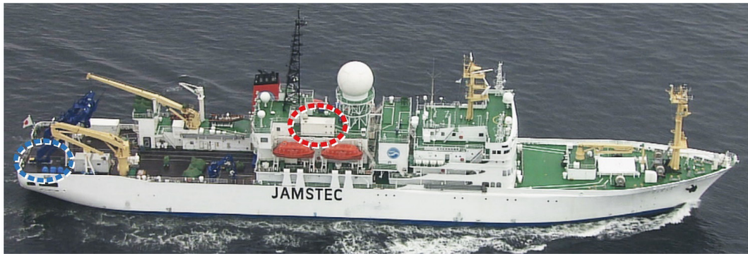
Fig. 1 Photo of the research vessel (R/V) “Mirai”. The blue and red broken circles indicate the locations where lidar systems were (are) installed: Blue is for special container including HSRL (see section 3), while red is for “Mirai lidar” in the radiosonde container (see section 4).
