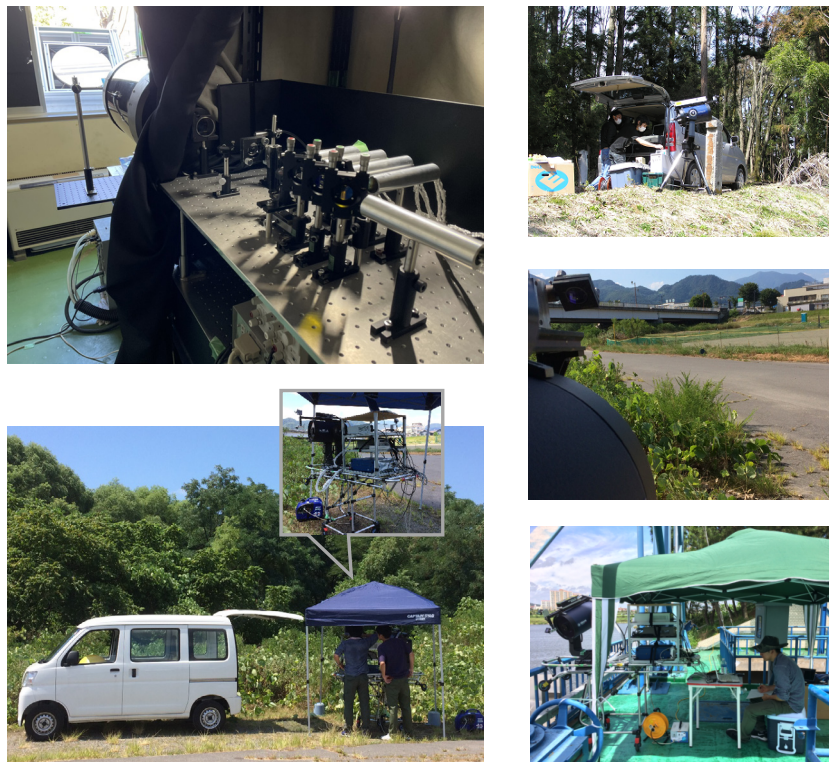
Fig. 4 Photos of the earth environmental sensing by the fluorescence lidar: Atmospheric aerosol (upper left), vegetation (lower left), pollen (upper right), waste-plastic and soil (middle right), and river water (lower right).
