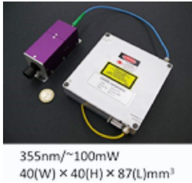
Fig. 5 Compact 355 nm laser module.
