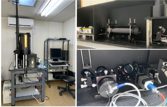
Fig. 3 Photographs of the AD-Net lidar in Tsukuba. (left) Overall view, (right top) transmitter, (right bottom) receiver.
