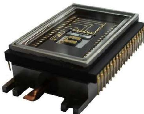
Figure 8 The detector with the ACCD chip housed in a thermo-controlled hermetically sealed package
