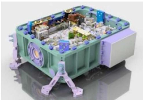
Figure 17. Preliminary design of the MERLIN laser source
