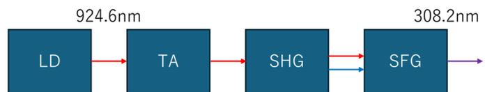
Fig.4 Block diagram of the diode laser base transmitter system.
