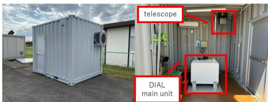
Fig. 2 The exterior of the ship-based water vapor and wind coherent lidar container (left) and its inside (right)
