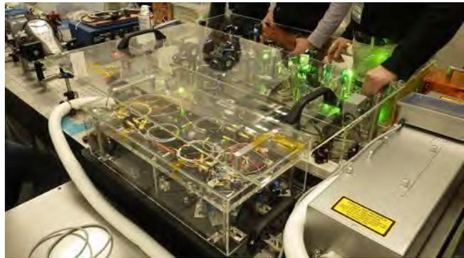
Fig. 1 Injection-locked Ti:Sapphire pulse laser system installed at the National Institute of Polar Research.
