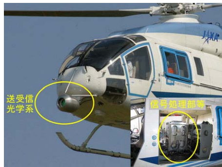
Fig. 8. MuPAL-ε with the lidar system installed
