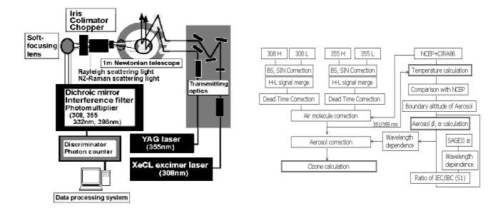
To get the pure backscatter signal, method to remove the background noise and the signal induced noise simultaneously was developed and applied. Also using the high/low channel combined method, the problem of dead time effect caused by the shortage of dynamic range of the system was solved. Figure 2 shows the flow chart of the signal and data processing
