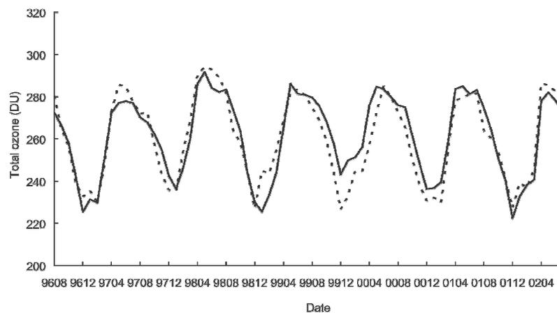
Fig.2: Year-to-year variation of total ozone over the subtropical western Pacific from EP\_TOMS (solid line) and the nudging chemical transport model with ECMWF data (dashed line). An area-weighted mean of  $15^{\circ}$ - $25^{\circ}N$ ,  $120^{\circ}$ - $150^{\circ}E$  was shown.
