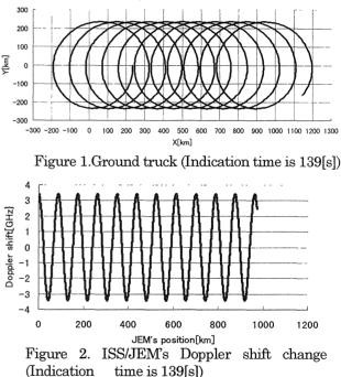
In general, the attitude of ISS/JEM isn't constant. So, it is necessary to evaluate how large the fluctuation of Doppler shift frequency caused by it will be. This is important when we select the bandwidths of amplifier and photo-mixer used in the heterodyne receiver. Fig.3 schematically shows a relation between ISS/JEM's attitude, X axis, Y axis and altitude. X corresponding to a rolling angle and Y a pitching angle are derivated as Eq. (2) and Eq. (3), respectively.
