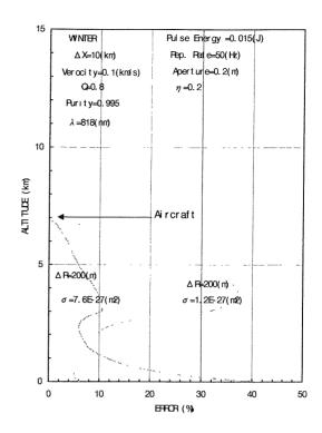
Fig. 2 Error simulation of the airborne water vapor DIAL
