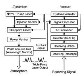
Fig. 1 Schematic diagram of the airborne water vapor DIAL
