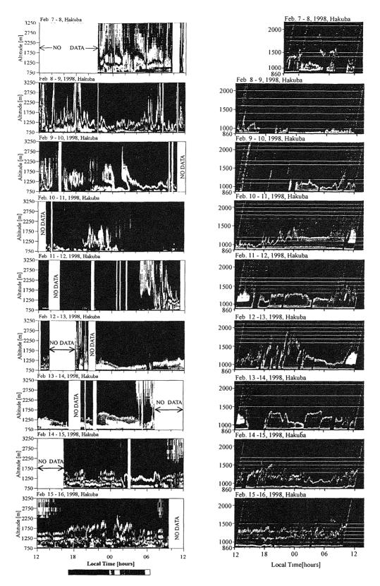
Fig.5 Time – height representations of the laser return signal intensity measured with bistatic imaging Lidar (left) and monostatic lidar (right) at Hakuba from noon Feb.7 to noon Feb.16, 1998
