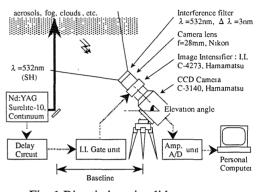
Fig. 1 Bistatic imaging lidar system
