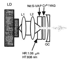
Fig. 1 Schematic diagram of the passively Q-switched Nd:S-VAP laser
