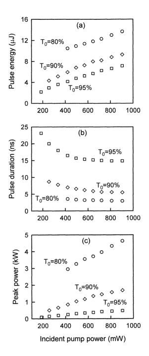
Fig. 2 Pulse parameters versus incident pump power for  $Cr^{4+}$ :YAG saturable absorbers of initial transmission  $T_0 = 80\%$ , 90% and 95%, respectively. (a) Pulse energy, (b) Pulse duration, (c) Peak power.
